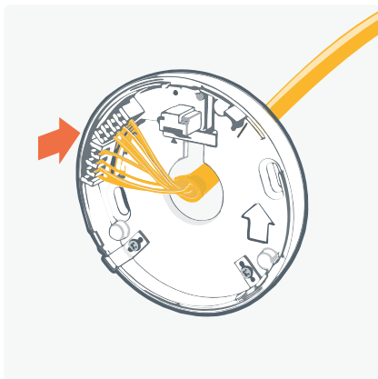
Figure 23 Punch down Ethernet cable
